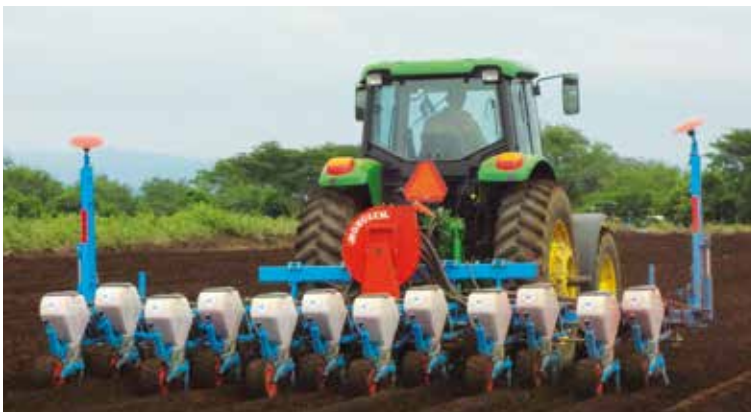
NC Classic V2 - 2x6 rij Twin-Row Dubbel frame star (6 rijen Twin-Row)
